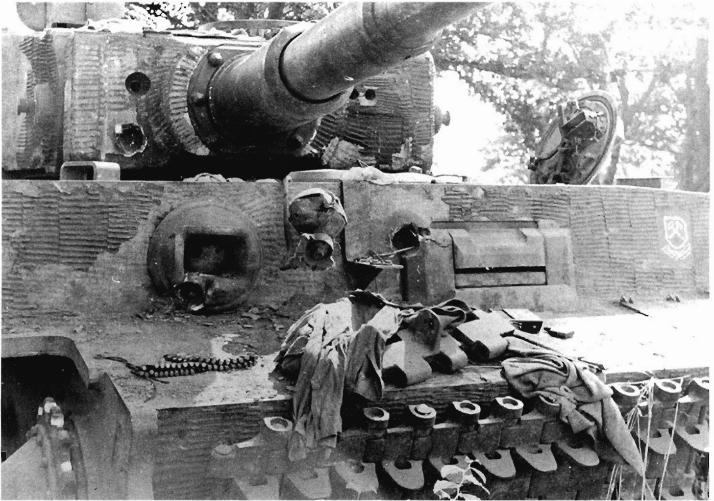
The frontal armor of this Tiger of the schwere SS-Panzer-Abteilung 101 successfully held up to the punishment from the opponent's anti-tank guns. (NA)
