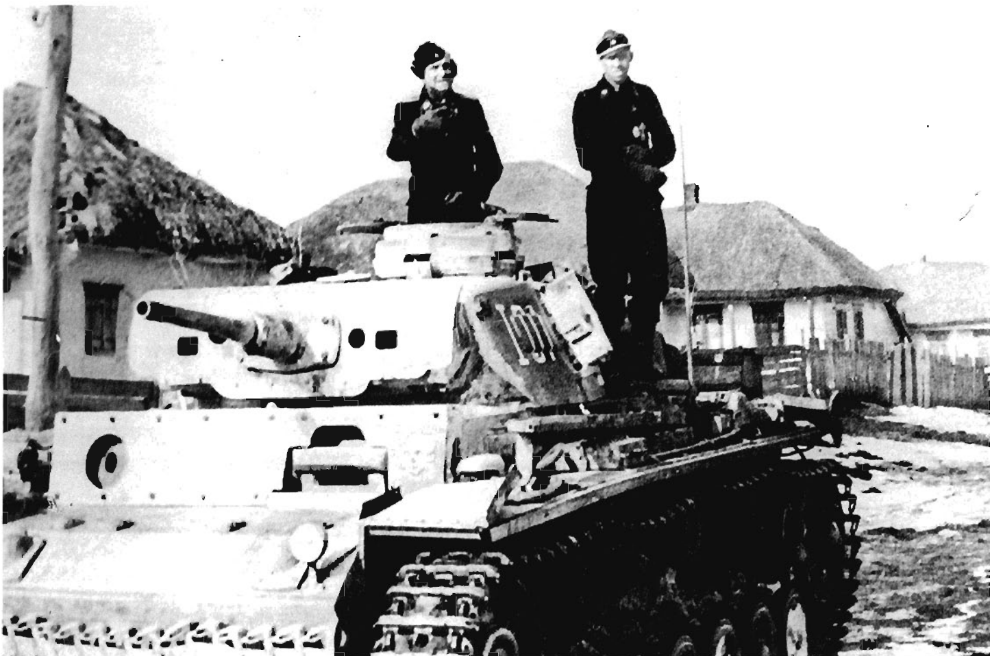
The Pz.Bef.Wg. Ausf.J belonging to the I.Abteilung/SS-Panzer-Regiment 3 had a pistol port for the radio operator instead of a machine gun ball mount. (HLD)
