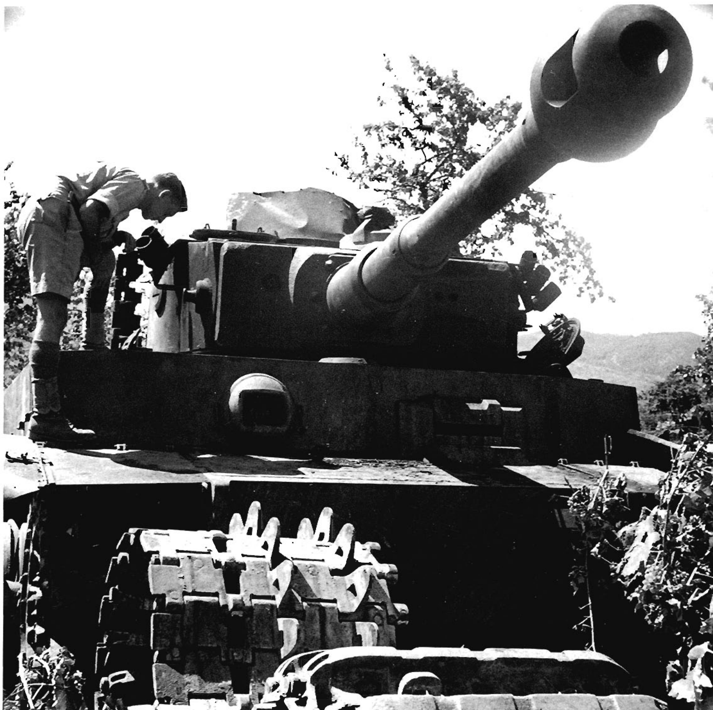
A Tiger from the 2.Kompanie/schwere Panzer-Abteilung 504 abandoned in Sicily after apparently losing the right track after hitting a mine. (TMM)
