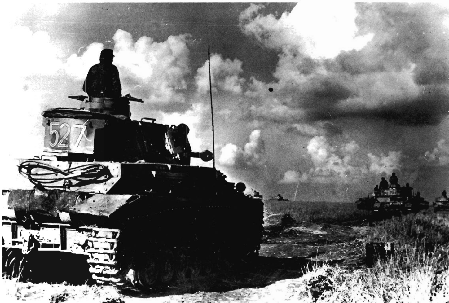
A Kompanie of Pz.Kpfw.IV Ausf. Gs advancing across a wheat field at the start of Operation Zitadelle . The last Pz.Kpfw.IV had not been outfitted with Schuerzen , although others in the lead have the additional protection against Russian anti-tank rifles. (BA)
