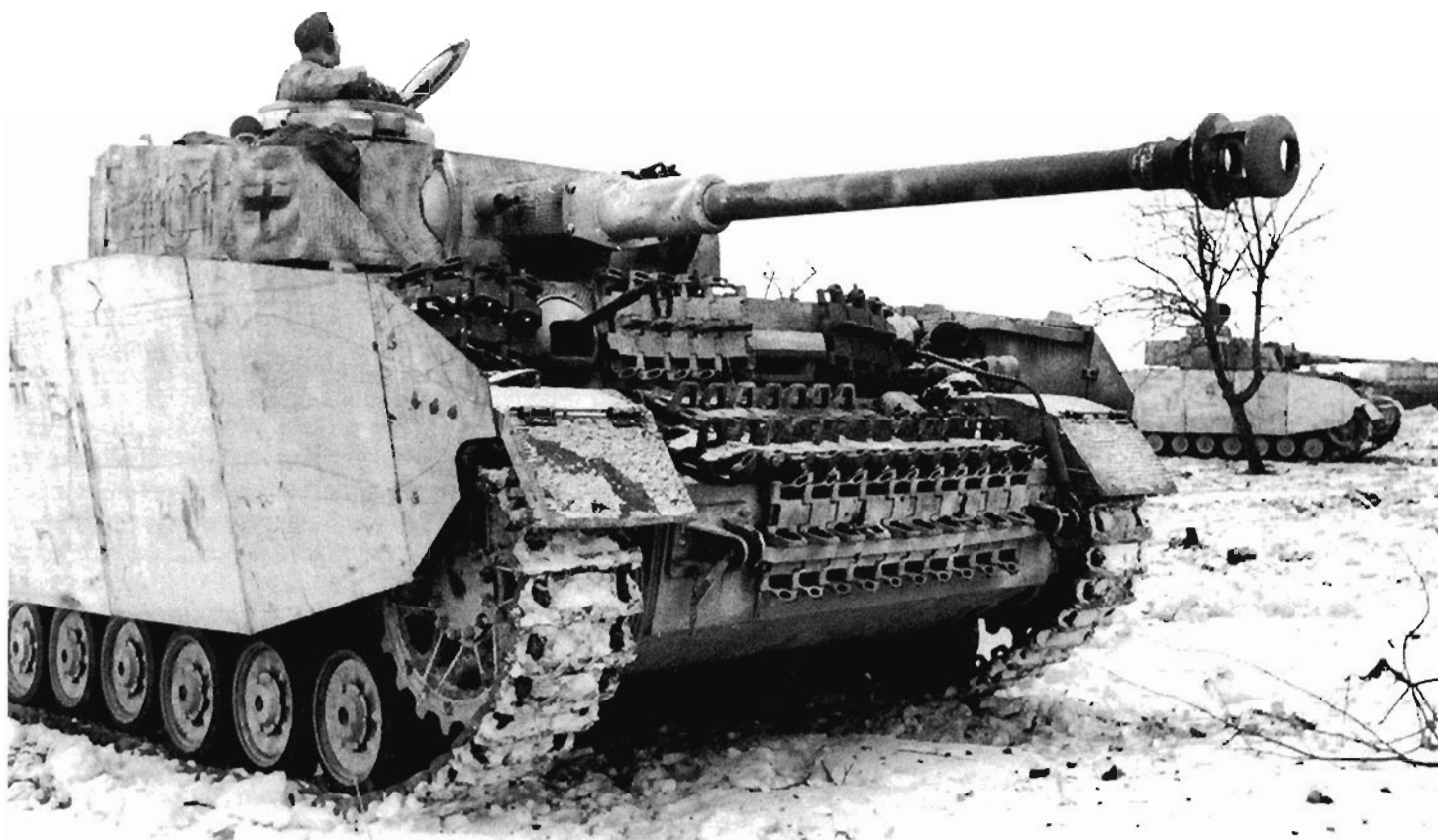
A row of Pz.Kpfw.IV Ausf.Hs on alert. The Schuerzen fasteners had been improved to prevent their being lost when encountering brush. (BA)
