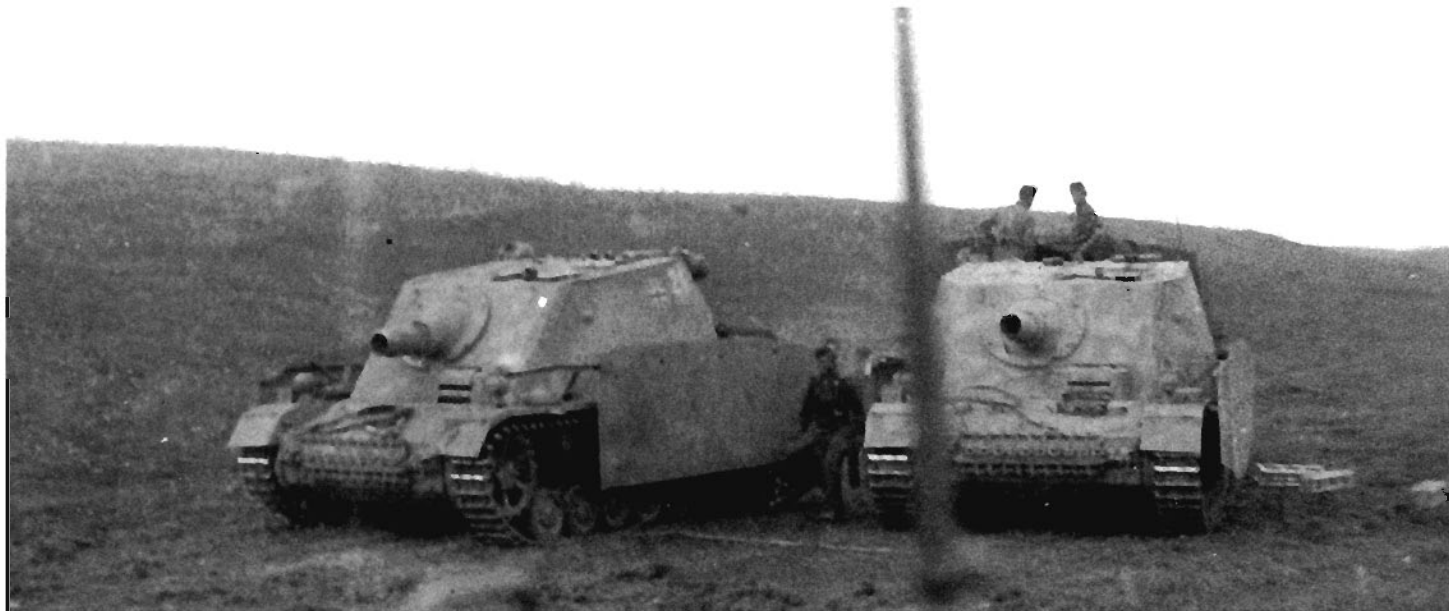
Two Sturmpanzers from Sturmpanzer-Abteilung 216 loading ammunition. The troops complained that the method of fastening the Schuerzen (side skirts) to the rails and fenders was inadequate to prevent their loss. (KHM)
